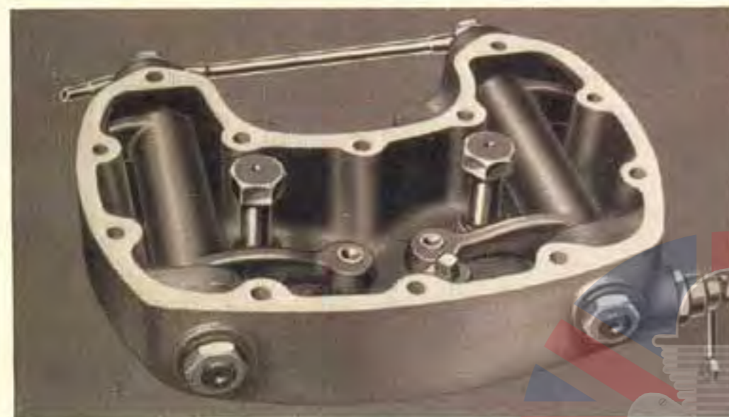
The photograph above of the totally enclosed overhead rocker gear with cover removed shows the pressure oil feed to the hollow rocker shafts on the 350 c.c. O.H.V. De Luxe and 500 c.c. O.H.V. models.
