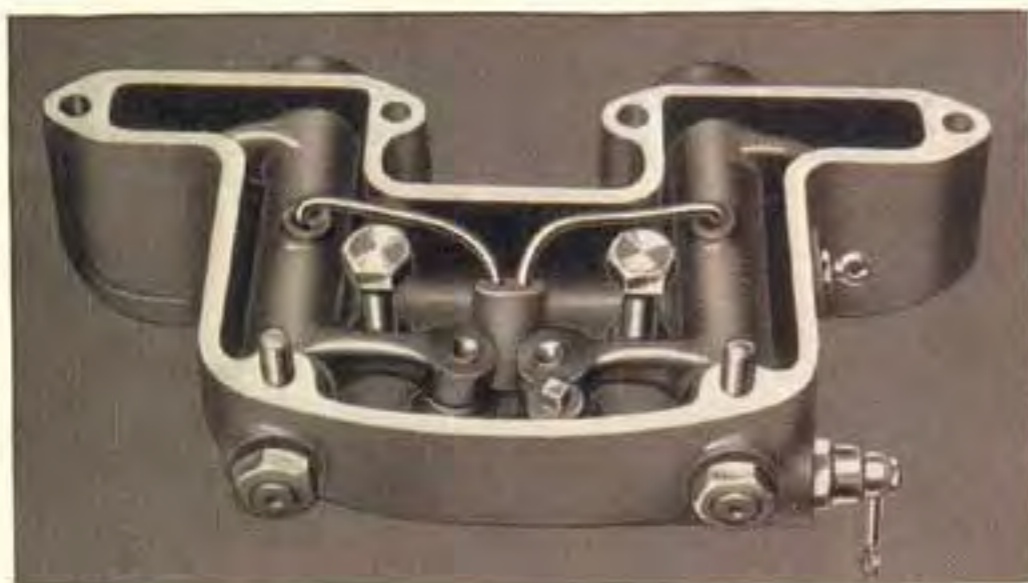
The picture below of the totally enclosed overhead rocker gear shows clearly the special oil distribution to the valve rockers.
